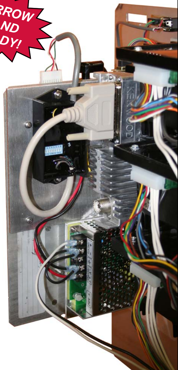
The GTS-5500 Siren/Radio Interface shown installed in a WHELEN® IPS-800 Cabinet.
